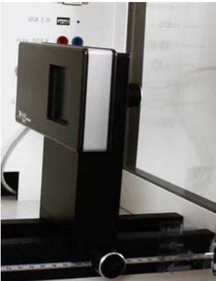
Fig. 4: X-ray sensor XRIS in a holder mounted on the optical bench of the X-ray unit
